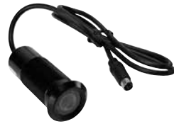
160610 Camera, O.D. 30 mm. L. 70 mm. Wide view angle, 130° diagonal.
